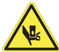
Warning sign: pinch-ing hazard
