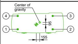
The floor construction has to be performed solid and free of vibration, e.g. concrete flooring C20/25 to C50/60 corresponding to DIN EN 206-1, according to the maximum values as specified in the textblock "Floor and building vibrations".
