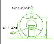
The climatic room conditions for all air-cooled CT system components are influenced by design room conditions (e.g. windows, large glass areas, building and room insulation, room size and volume, etc.) and must be observed in the case of a new or existing air conditioning system in the examination room.
