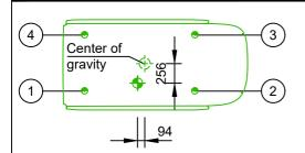
The floor construction has to be performed solid and free of vibration, e.g. concrete flooring C20/25 to C50/60 corresponding to DIN EN 206-1, according to the maximum values as specified in the textblock "Floor and building vibrations".
