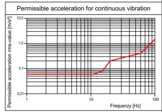
Any transient vibration (shocks) has to be less than  $0.5 \text{ m/s}^2$  peak-to-peak in the time domain. The vibrations have to be measured with a sampling rate of 1000 Hz.
