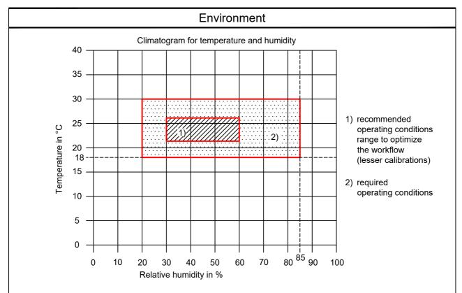
The climatograms shows the permissible temperature ranges.
