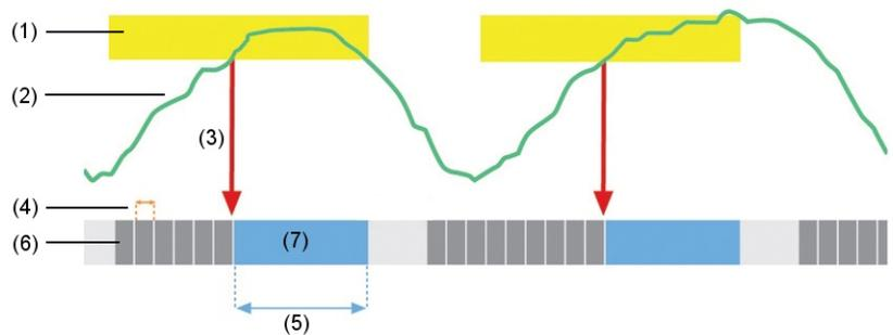
**Imaging phase of navigator-triggered sequence.** After completing one block of the imaging sequence, the navigator is repeated until the next suitable respiratory phase is located. No triggers are generated during inspiration (acceptance window is interrupted).
