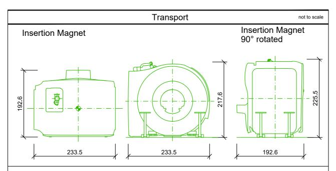
Min. transport opening in the wall: W = 200 cm / H = 240 cm Min. transport opening in the ceiling: L = 200 cm / W = 245 cm
