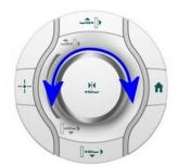
1 Keep the jog wheel turned to move the patient table up/into or down/out of the magnet bore.
