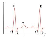
The characteristic QRS complex of the ECG signal is used as a trigger signal. Simultaneous acquisition and overlaying of the orthogonal leads (vector cardiography) is used to minimize triggering errors due to gradient switching and the magneto-hydrodynamic effect (i.e. excess T-wave amplitude).
