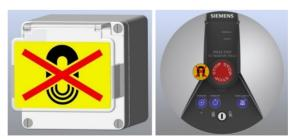
After the **Magnet Stop** switch has been pressed, an alarm is triggered at the alarm box. The **WARNING** LED will light up and an alarm signal will sound.
