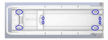
The coil sockets are located at the head end and the foot end of the patient table. For more information concerning the occupation of the coil sockets, see: **Coil operator manual**
