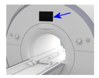
The display is located above the magnet bore opening at the front of the magnet cover. Optionally, at the back of the magnet, a second display can be installed for the additional control unit.
